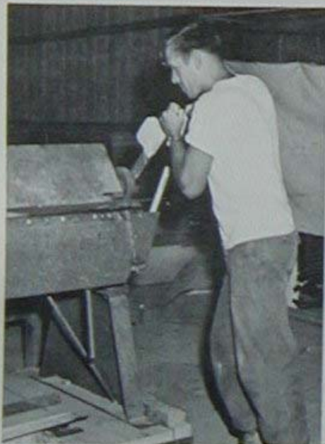
SW3 Bert Noles from Sarasota, Florida, bends sheet metal on the break.
